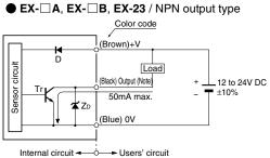
Note: The emitter of thru-beam type sensor does not incorporate the output.
